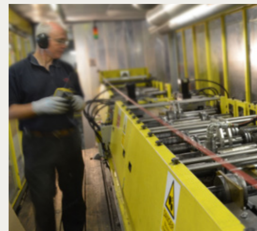
Splitter Line A bespoke piece of machinery at our product centre for automated manufacturer of splitters.
