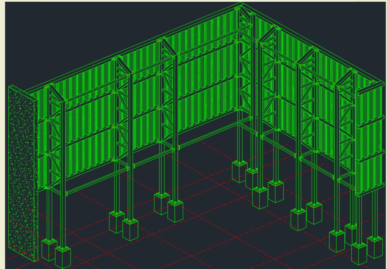
Our design team prepared 3D images and modelling for the required louvre screening along with structural and windload calculations.
